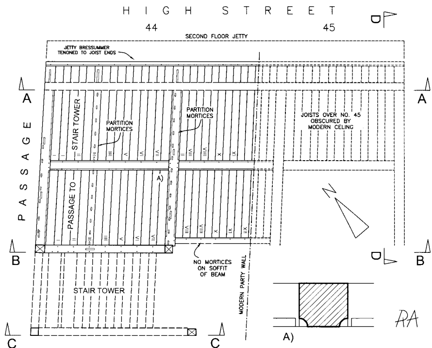
REFLECTED FIRST FLOOR FRAMING SHOWING JOISTS AND BEAMS ABOVE GROUND FLOOR SHOP
